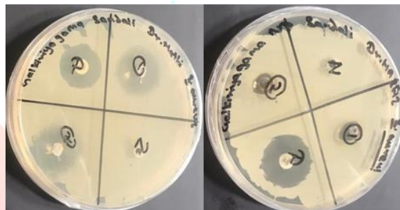
Figure 12: Zones of inhibition (ZOI) of S.aureus in Galkiriyagama water extract (left) and AgNPs (right).
