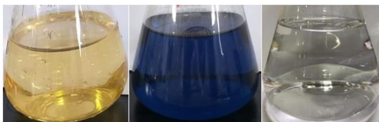
Figure 8: Colour change from pale yellow to blue after the addition of starch and blue to colorless at endpoint.
